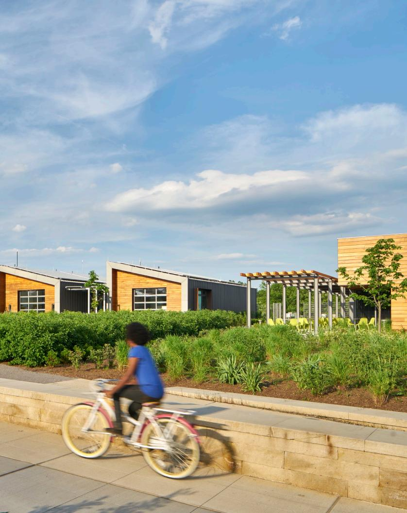
**Design-integrated Rainwater Flows**— Rainwater runoff is captured along the base of the wall and raingarden patches, and then flows by gravity to a stilling well at the base of a large tree beyond.
